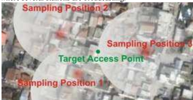
Figure 11: Triangulation of a known Target AP
